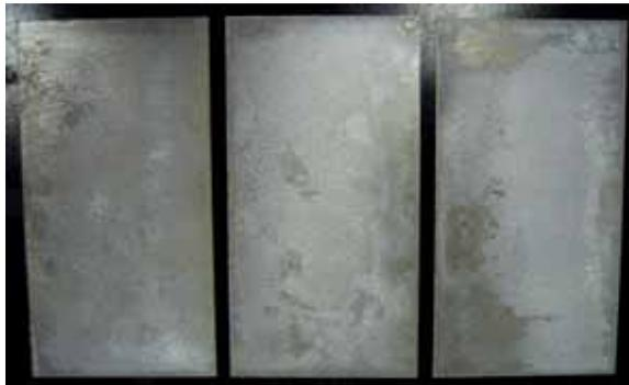
**Fig. 7.** Results of specimen 2 with various concentration of formic acid after black tarnish test; concentration of formic acid from left to right: 12.5, 25, and 50%.
